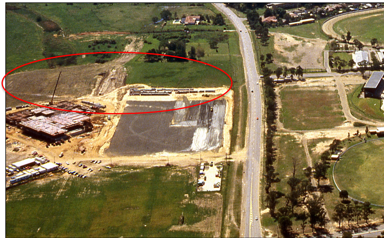
Photograph 2. 1983 Panthers Construction: filled and disturbed areas circled
